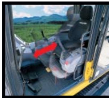
Seat Sliding Amount: 340 mm 13.4", increased 120 mm 4.7"
