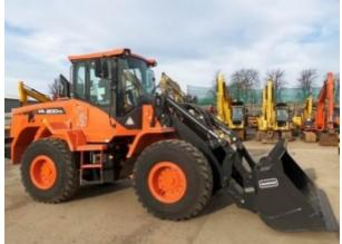
The parallel-lift linkage system keeps other products. the job device level as it is raised, a benefit when lifting pallets and also other loads that should stay level. The high pressure gas injection engine delivers outstanding digging power for taking on difficult materials. Outstanding tractive power allows much easier container loading in hard products. Two selectable procedure modes enable the operator to stabilize efficiency as well as power.
