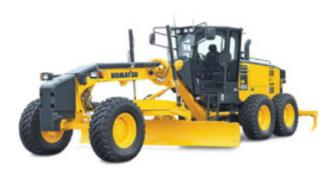
• Engine: Komatsu SAA6D107E-1, EPA Tier 3 certified, turbocharged and air-to-air aftercooled, standard VHPC, 145-218 net horsepower • Fuel line pre-filter • Hood-sides for engine compartment • Air intake extension
