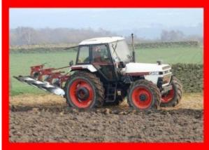
Mechanical: Chassis: 4x2 2WD Differential lock: standard Steering: hydrostatic power Brakes: drum Cab: Cab standard. Hydraulics: Type: open center Pressure: 2550 psi [175.8 bar] Valves: 1 Pump flow: 7 gpm [26.5 lpm] Steering flow: 2 gpm [7.6 lpm]
