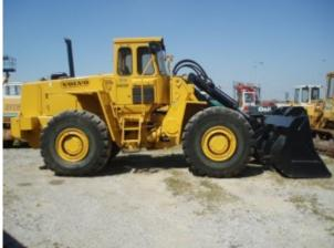
The parallel link arm system showcased high breakout moment in the leading location while maintaining power in all other placements integrated with very friendly parallel motion. The disign of the arm system additionally paid for the driver superb ahead visibility.
