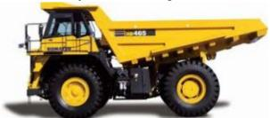
**Power mode** Great productivity can be attained by taking full advan- tage of high output power. It is appropriate for job sites where large production on an uphill haul is required. Economy mode (Variable horsepower control) Engine speeds of the maximum output, downshift, and upshift are set to a lower level. It is suitable for light work on a flat haul.
