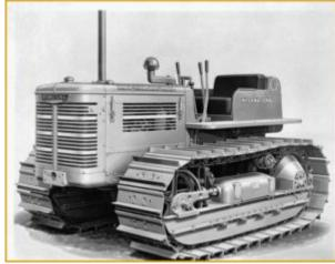
The International T-6 and TD-6 were new small caterpillars of International, introduced earlier by the styling theme on the TD-18th The original models of the whole crawler line used bonnet side walls with a horizontal silver bar on the side walls on the grille horizontal correspond silver bullion. Somewhere around 1950 the side walls were dropped (or made optional), and the grid was all painted red.
