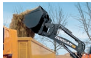
Parallel kinematics (Tool Carrier) Provides maximum force for high reach and a constant tilt angle of the attachment at any height.
