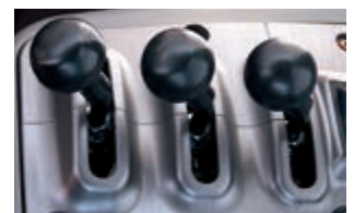
Fingertip control 3-lever control for lift arm, bucket and 3rd circuit. FNR switch for changing travel direction as well as kick-down, return to dig, lift arm raise kick-out and floating mode.
