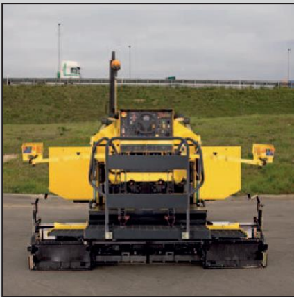
The working width of 2.6 m is achieved with the basic screed. Step-by-step extension up to 4 m is possible.
