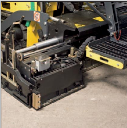
Particularly advantageous on narrow construction sites: the side plates can be adjusted from behind as well using the offset crank handle.
