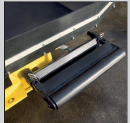
The truck push rollers are raised with the hopper wings to save space; they can be adjusted to the size of truck.
