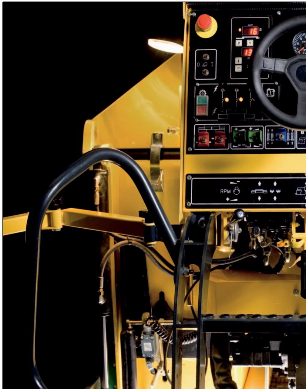
The main operating panel on the BF 223 C with electric screed heating.
