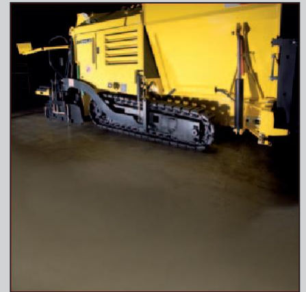
200 mm wide, screwed-on rubber floor plates reliably transfer forces even on loose subbases.
