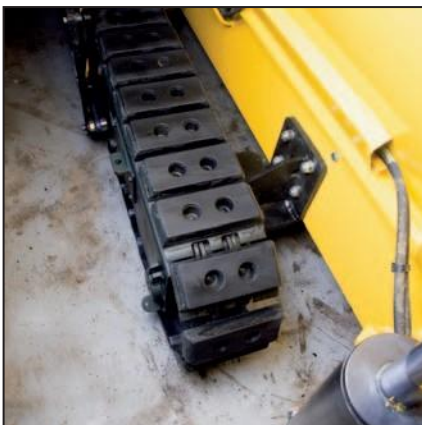
Bolt-on rubber floor plates – this increases traction, is kinder to kerbs and simplifies maintenance.
