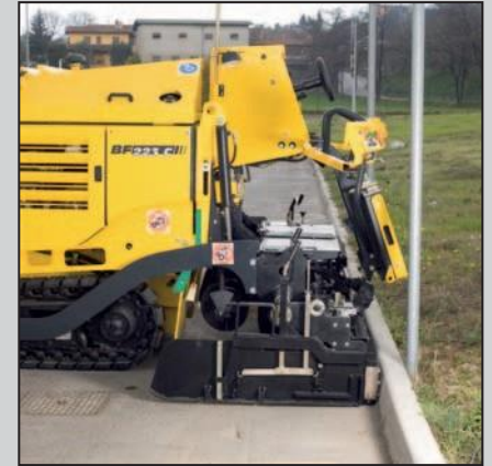
With a fully folding operator's platform, the screed can work "against the wall", e.g. in workshops and multi-storey car parks.
