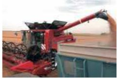
▲ Huge capacity grain tank. Up to 10,500 litre grain tank with electrically controlled quick-folding extensions that don't require tools. The tank is completely closed in the folded down position.
