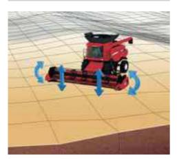
▲ Perfect ground hugging. The Terrain Tracker header control system keeps the header parallel to the ground in undulating conditions.
