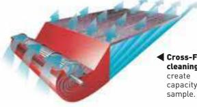
Cross-Flow™ fan and X-tra Force™ cleaning system. The perfect match to create powerful dynamics for high capacity cleaning and excellent crop sample.
