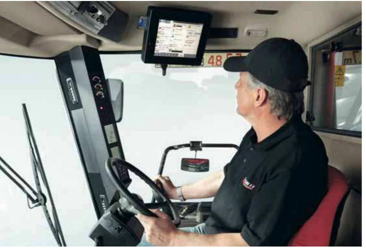
**Propulsion lever puts full control in your hands.** Header height resume, header raise/lower and tilt, reel raise/lower and fore/aft, unloader swing and engage, emergency feeder/header shutoff, shift functions (headland, draper side to side tilt, real fore/aft, guidance side shift).
