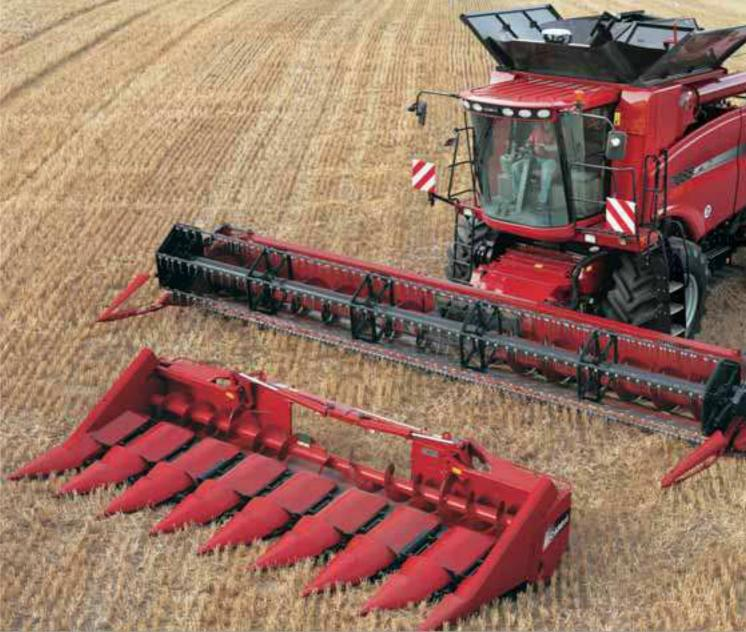
**Axial-Flow rotor - the heart of the process.** Constant pitch impeller for top quality grain, crop adaptability and highest performance per hectare. **Greater profit potential with premiumquality grain.** Case IH Axial-Flow design provides a smooth, gentle rubbing action on the crop. The market leader for grain quality. **Optimised concaves.** 156° of concave wrap for really high throughputs.
