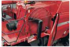
▲ Self-cleaning engine air screen. Hydraulic-driven rotating wand, evacuation fan, tree branch guard and internal brush for use with chopping corn headers.
