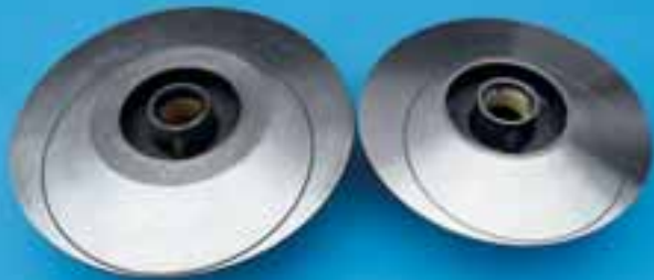
Larger-diameter rotor pulley Previous rotor pulley
