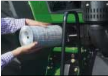
The cab air filter is located on the right side of the cab. You can remove and replace the filter from the ground. Air intake is from above the door, away from dust and debris.
