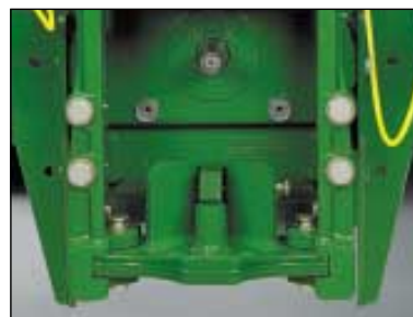
The high clearance piton fix type hitch provides the strength and security required for transport applications.
