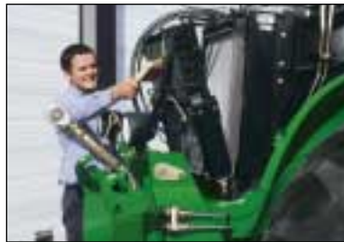
The radiator flips forward for easy cleaning. Strong latches hold it securely while you're operating the tractor.
