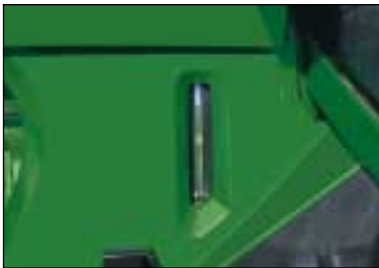
Check the engine coolant level at a glance with the sight glass. It's located at the front of the tractor near the fuel fill for quick service.
