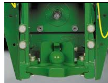
The ball hitch is useful in applications where a tractor is dedicated to implements such as sprayers or liquid manure application.
