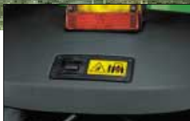
Remote switches for the rear hitch make it easy to hook up implements from the ground. A slower raise/lower rate keeps you safe.
