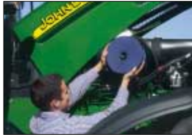
The engine air filter can be replaced from the ground. Air flows freely through the large grill screen and side louvres for good intake and cooling.
