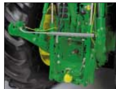
The hydraulic push back, pick-up hitch gives you an excellent view for easy coupling and can be pushed into the soil to recover sunken trailers.
