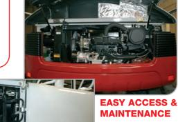
Service access on the machine is simple, with access points to the battery, air and fuel filters, engine and radiator.
